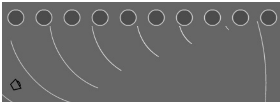
그림 3 - The reflected sound waves from repetitive elements can sometimes be detected as an audible 'pinging' sound
