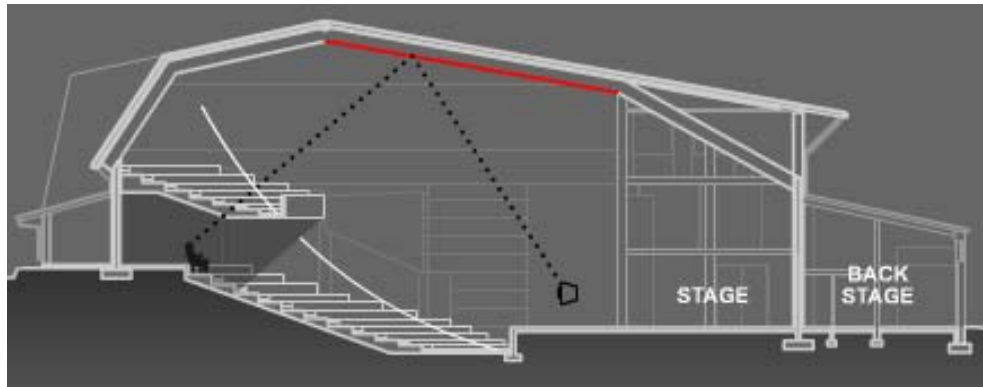
그림 5 - A acoustic dead spot can occur where the direct sound is not clearly audible and no secondary reflections are heard to reinforce it.
