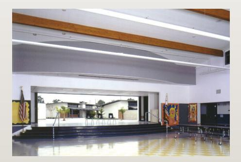
CLERESTORY WINDOWS AND SHADING ARE COMBINED TO PROVIDE PROPER AMOUNTS OF DAYLIGHT TO THE CLASSROOMS.
