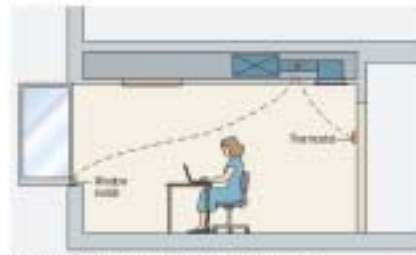
FIGURE 6. An office HVAC control interface of with a window switch
