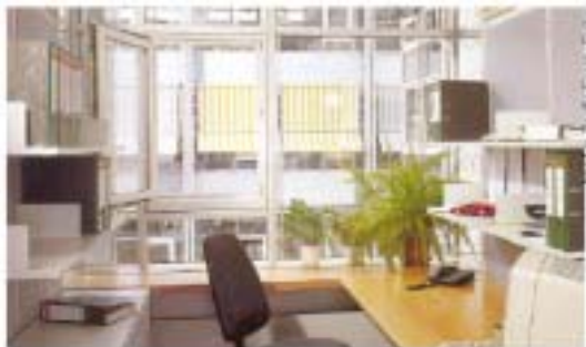
Buildings with operable windows exhibit fewer symptoms of sick-building syndrome.
