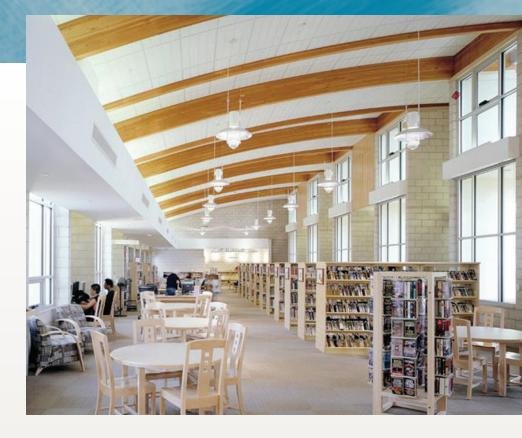
Dimmable ballasts, photocells, and occupancy sensors are part of the electric lighting system, and integrate the electric lights with the daylight to ensure target light levels are provided throughout the day and night.
