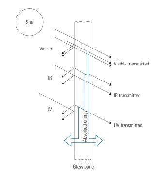
systems with high values of Tv (0.7 to 0.9) provide lots of natural light and good vision, but they can also be a source of unwanted glare if not properly controlled. Systems with lower values of Tv (less than 0.4) can be visually distorting and quite gloomy on cloudy days.
