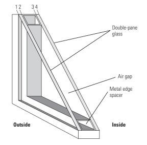
mates, buildings with HVAC systems that are frequently in cooling mode when the outdoor temperature is lower than the indoor air temperature may gain little benefit from installing insulated glass. However, a similar building in a cooler climate where significant amounts of heating energy are required probably would benefit from insulated glass.
