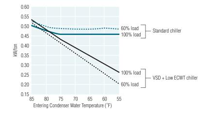
combination of low entering condenser water temperature (ECWT) capability and a VSD-driven compressor can provide an average of 30 percent annual energy savings and up to 75 percent savings under light load conditions, compared to a fixed-speed, fixed-condensing water temperature chiller.
