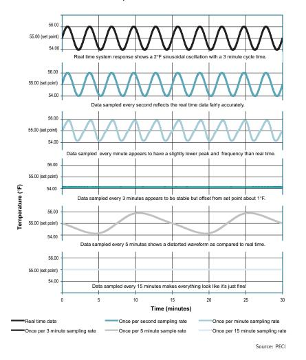
minutes at the most. Control points may wander around during the start-up process as the various control loops interact and attempt to meet the load, but the deviations should not be extreme.<sup>3</sup> The peaks in the oscillations should drop in magnitude with each cycle as illustrated in **Figure 10**, page 28.
