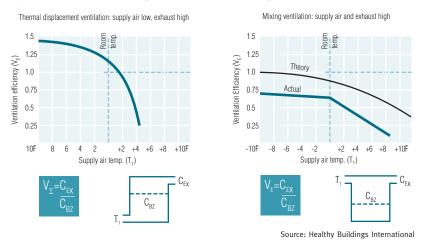
perspective, ventilation or "air-change" effectiveness is defined as the ratio of contaminant concentration in the return air to the contaminant concentration in the breathing zone of the room.
